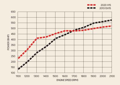
Braking power is available where you need it most, at lower rpms, providing better drivability and extending service brake life.
