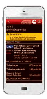
A notification based on the most probable cause is sent instantly to you via email or the free Connected Diagnostics mobile app, so you know exactly what action to take. That reduces guesswork and allows operators to safely proceed on their trip with the knowledge of the probable cause and information on when service can wait or if it needs to be performed immediately.
