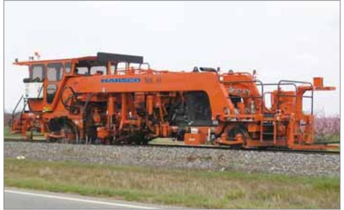
Cummins powered Harsco tamping machine
