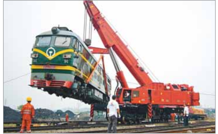
World's largest rail crane powered by a Cummins QSB
