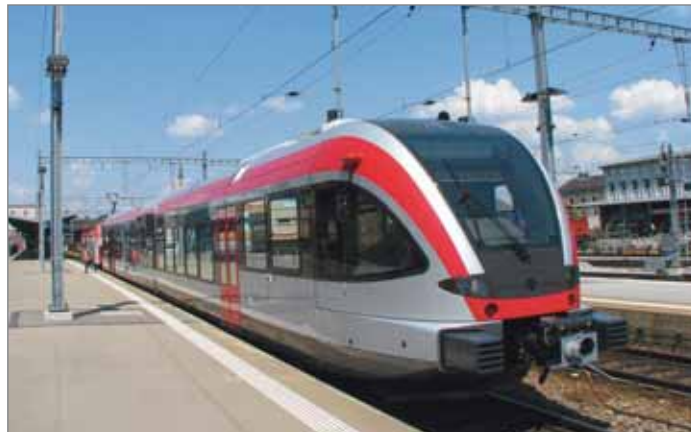
QSM11 powered diesel multiple unit
