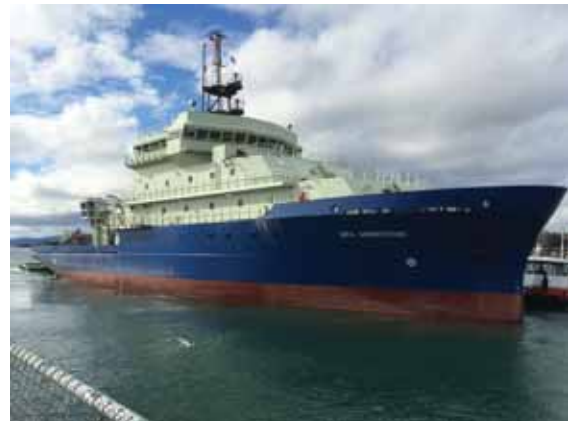
Research vessel powered by four Cummins QSK38 diesel electric generators (U.S. Navy)
