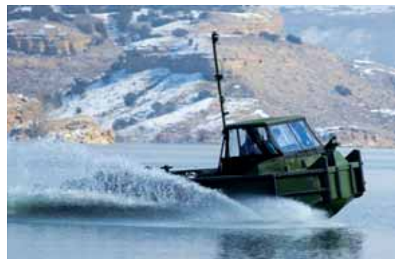
From top: over-the-horizon boat powered by one Cummins QSB6.7 480 hp (U.S. Coast Guard); harbour patrol boats powered by two Cummins QSB6.7 425 hp (U.S. Navy); bridge erection boat powered by two Cummins QSB6.7 250 hp (U.S. Army)
