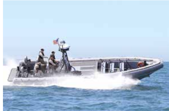
Rigid hulled inflatable boat (RIB) powered by two Cummins QSB6.7 380 hp (U.S. Navy | image courtesy of Willard Marine)
