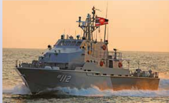
Patrol boat powered by three Cummins KTA50 1800 hp (Royal Thai Navy)
