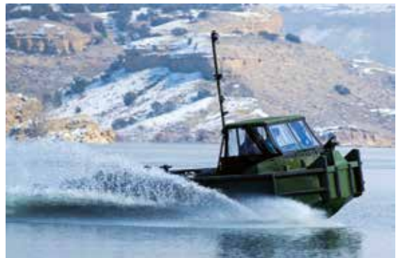
From top: over-the-horizon boat powered by one Cummins QSB6.7 480 hp (U.S. Coast Guard); harbour patrol boats powered by two Cummins QSB6.7 425 hp (U.S. Navy); bridge erection boat powered by two Cummins QSB6.7 250 hp (U.S. Army)
