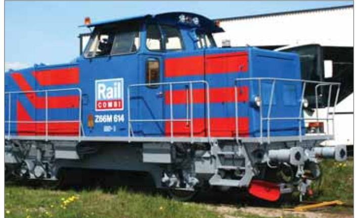
QSX15 powered shunting locomotive in Scandinavia
