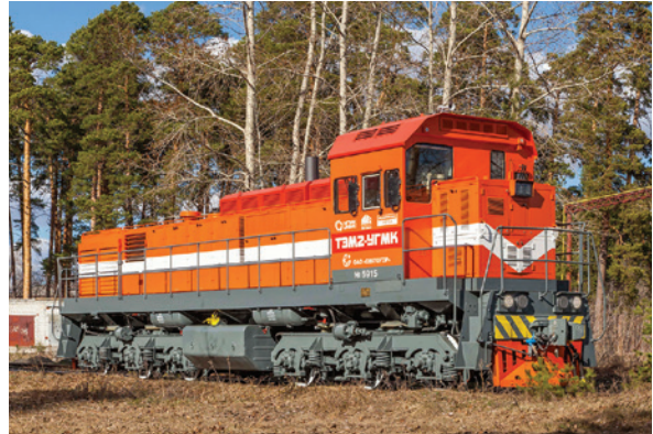
TEM2-UMMC DE Loco powered by Cummins QST30 L2 Engine
