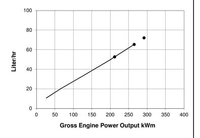
Rating Conditions: Ratings are in accordance with ISO 15550 and ISO 8528-5 reference conditions; air pressure at 100 kPa (29.61 in Hg), air temperature 25 ℃ (77 °F), and 30% relative humidity. The fuel consumption data is based on No. 2 diesel fuel weight at 0.85 kg/liter (7.001 lb/U.S. gal).
