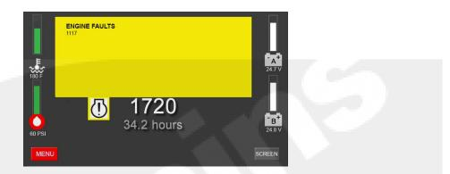
Figure 2-6 Yellow warning indicator ISO symbol and overlay box
