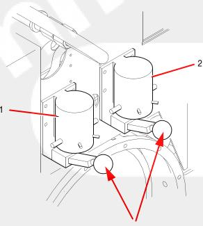
Battery contactor levers
