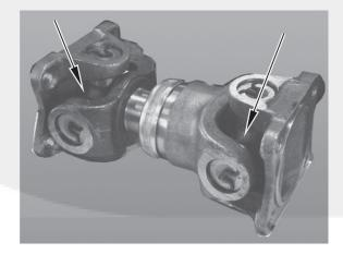
Figure 3-2 Drive shaft universal joint grease fittings
