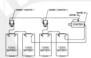
Figure 3-3 Series battery connection 24 VDC
