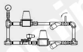
Figure 4-1 Water Bypass Valves
