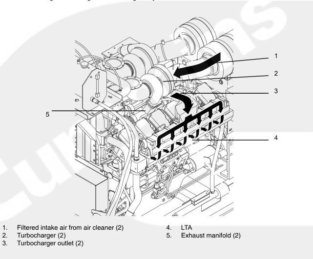
Figure 2-18 Engine air intake and LTA flow diagram (typical)
