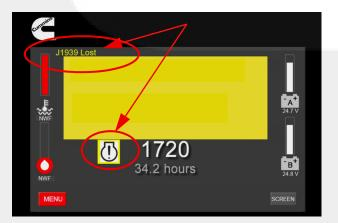
Figure 2-7 Loss of J1939 communications
