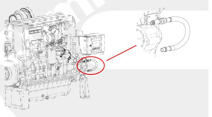
Figure 3-6 VSPLC pressure sensing connection
