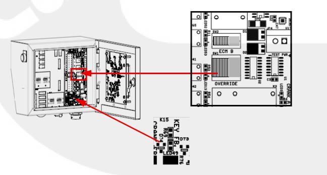
Figure 4-2 FPDP override switch
