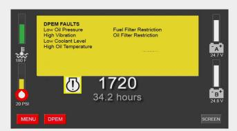
Figure 2-15 DPEM fault screen (sample)
