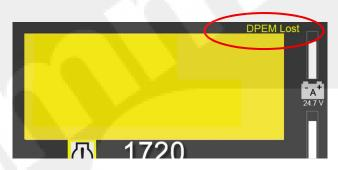
Figure 2-16 DPEM lost fault screen (sample)
