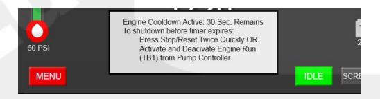
Figure 4-20 Engine/turbocharger cool down
