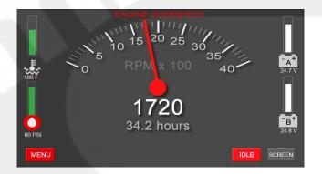
Figure 2-11 Overspeed warning indicator
