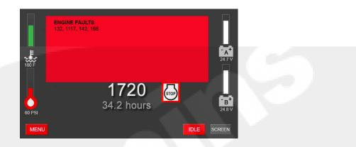
Figure 2-10 Red warning indicator ISO symbol and overlay box
