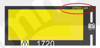
Figure 2-16 DPEM lost fault screen (sample)
