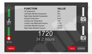
Figure 4-5 Analog Values overlay (electronic engine)
