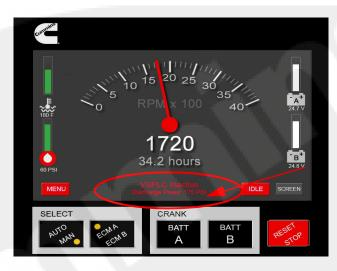
Figure 2-14 VSPLC inactive screen - red (sample)
