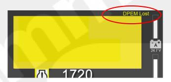
Figure 2-16 DPEM lost fault screen (sample)
