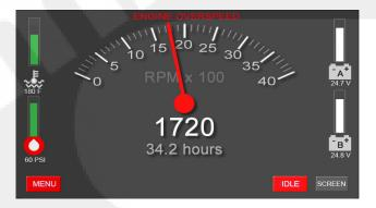
Figure 2-11 Overspeed warning indicator
