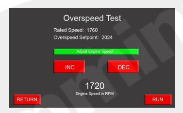
Figure 4-12 Overspeed Test screen
