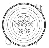
SAE J1936 standard connections are made as shown here.
