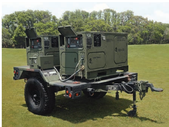
Two AMMPS units mounted on a trailer. Paralleling them is easy. Photo credit: U.S. Army.
