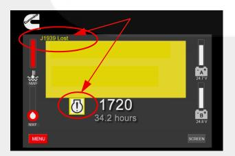
Figure 2-7 Loss of J1939 communications
