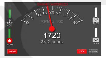
Figure 2-11 Overspeed warning indicator
