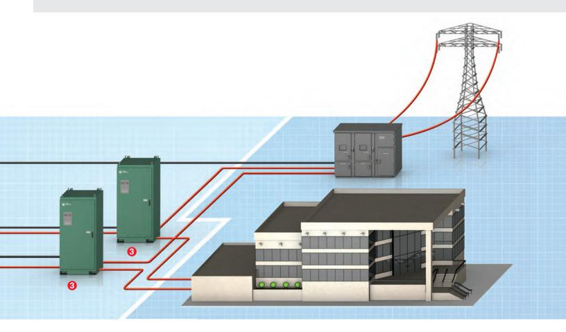
**3 Transfer switches.** Cummins automatic transfer switches feature PowerCommand control technology for easy operation and robust, high-contact-force design to withstand thousands of switching cycles. A full line of standard switches is available from 40 to 4,000 amps for the entire range of power systems with common bus communication language. Custom switches are available for unique project requirements.
