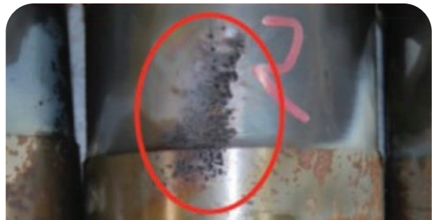
Erosion of cylinder liner outer surface which can lead to coolant contamination of oil.
