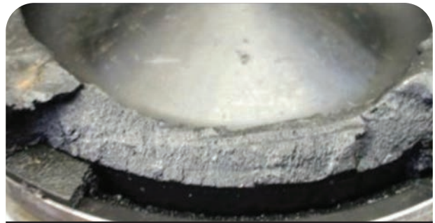
Non-genuine piston shows debond that could potentially lead to engine failure.
