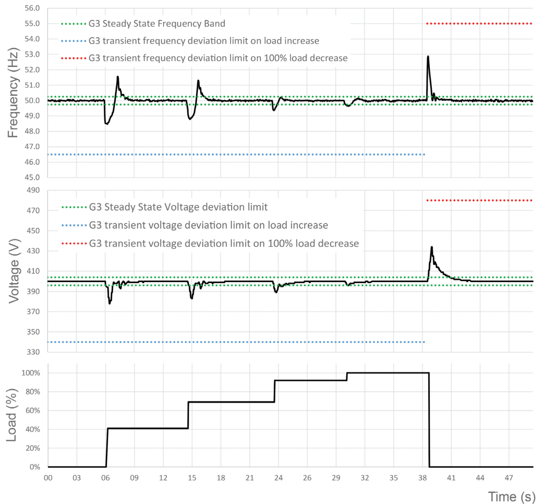
Figure 3. Extract of a transient test performed in the field on an engine with a BMEP of 1951 kPa using a purely resistive load bank (power factor = 1)
