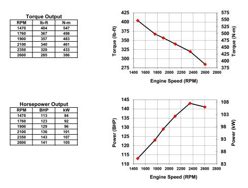
All data is based on the engine operating with a fuel system, water pump, lubricating oil pump, air cleaner, and alternator. The fan, optional equipment, and driven components are not included. Data is based on operation at SAE standard J1349 conditions of 300 ft. (91.4 m) altitude, 29.61 in. (752 mm) Hg dry barometer, and 77 °F (25 °C) intake air temperature, using No.2 diesel fuel only.
