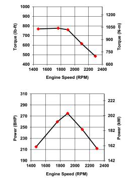
Horsepower Output BHP RPM kW 1470 215 160 1760 260 194 1900 275 205 2100 246 183 212 2300 158
