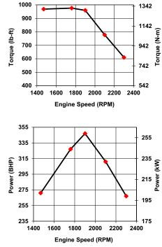
All data is based on the engine operating with a fuel system, water pump, lubricating oil pump, air cleaner, and alternator. The fan, optional equipment, and driven components are not included. Data is based on operation at SAE standard J1349 conditions of 300 ft.
