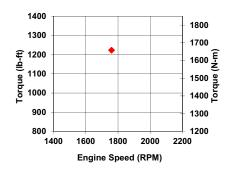
**Horsepower Output** RPM BHP kW 1760 410 306
