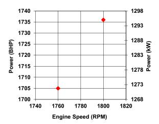
All data is based on the engine operating with a fuel system, water pump, lubricating oil pump, air cleaner, and alternator. The fan, optional equipment, and driven components are not included. Data is based on operation at SAE standard J1349 conditions of 300 ft. (91.4 m) altitude, 29.61 in. (752 mm) Hg dry barometer, and 77 °F (25 °C) intake air temperature, using No.2 diesel fuel only.
