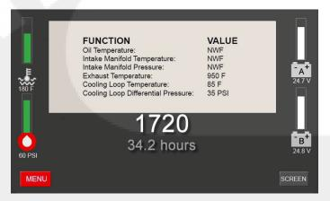
Figure 4-5 Analog Values overlay (mechanical engine)
