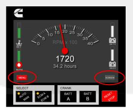
Figure 4-4 FPDP User Interface screen (mechanical engine)
