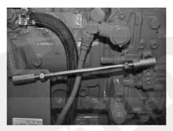
Figure 5-4 Fire pump drive engine linkage rod
