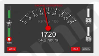
Figure 2-5 Overspeed warning indicator
