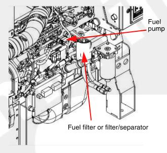
Figure 5-5 Typical fuel pumps and filters
