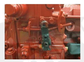
Figure 5-3 Fire pump drive engine threaded linkage rod
