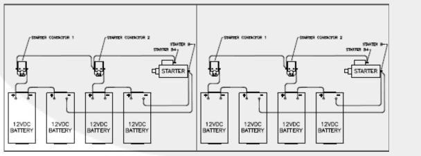
Figure 3-4 Series battery connection 24 VDC
