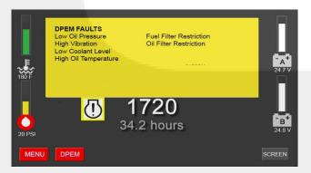
Figure 2-6 DPEM fault screen (sample)
