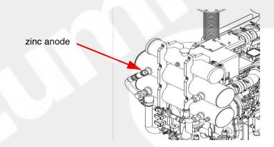
Figure 5-8 Raw water zinc anode (typical)
