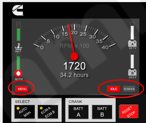
Figure 4-4 FPDP User Interface screen (electronic engine)
