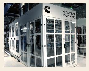
"Cummins technology powers the largest PEM electrolyser in operation in the world. Installed at the Air Liquide hydrogen production facility in Becancour, Quebec, the 20 MW Cummins electrolyser system can produce over 3,000 tons of hydrogen annually using clean hydropower. The modular and scalable electrolyser platform addresses utility-scale hydrogen production."
