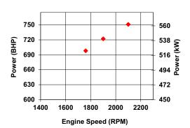
All data is based on the engine operating with a fuel system, water pump, lubricating oil pump, air cleaner, and alternator. The fan, optional equipment, and driven components are not included. Data is based on operation at SAE standard J1349 conditions of 300 ft. (91.4 m) altitude, 29.61 in. (752 mm) Hg dry barometer, and 77 °F (25 °C) intake air temperature, using No.2 diesel fuel only.
