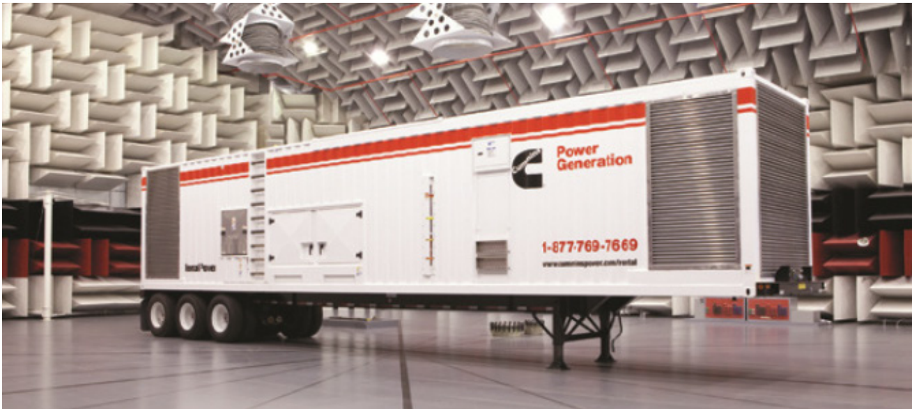
FIGURE 2 Inside view of the Hemi-anechoic chamber (part of ATC) with a rental generator set (trailer mounted container) which is 48 feet long, 13 feet high, and 8 feet wide.
