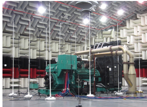
FIGURE 3 Noise measurement set up with 2250 kW capacity generator set and 59 microphones.
