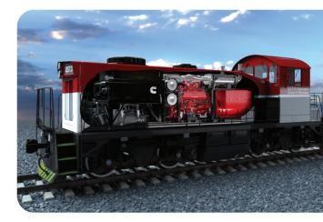
The Cummins QST30 Tier 4 Power Module is designed for ease of installation into multiple locomotive models. We preassemble the entire unit, including the engine, alternator, air intake, and exhaust, on a base skid. A separate cooling package is mounted directly to the locomotive frame with plumbing to and from the engine.
